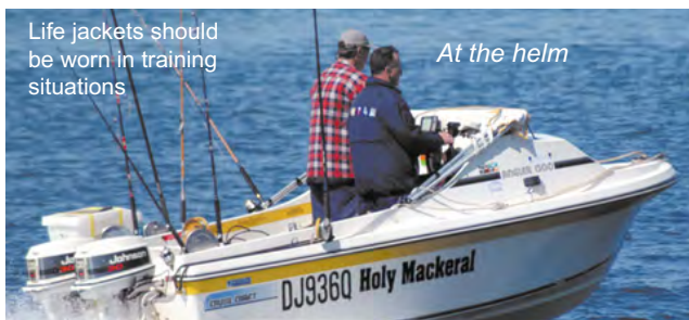
Figure 13.5 Twin engine boat "on the plane". Turn the wheel to port and the boat turns to port.
