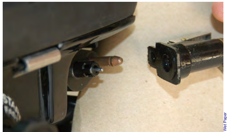
Figure 21.3 Make sure all fuel line connections are spotless.
