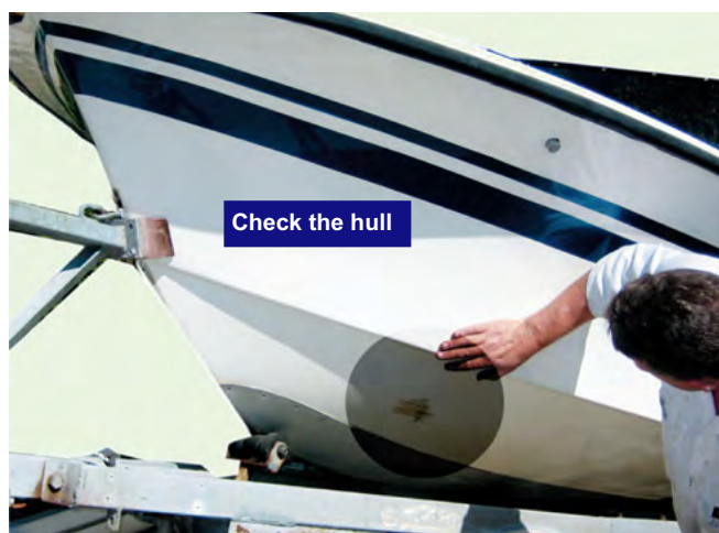
Figure 20.1 Inspect the hull for damage.
