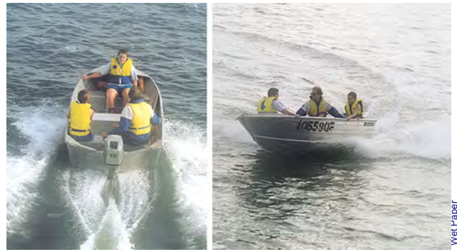
Figure 36.1 Correct seating for on the plane
