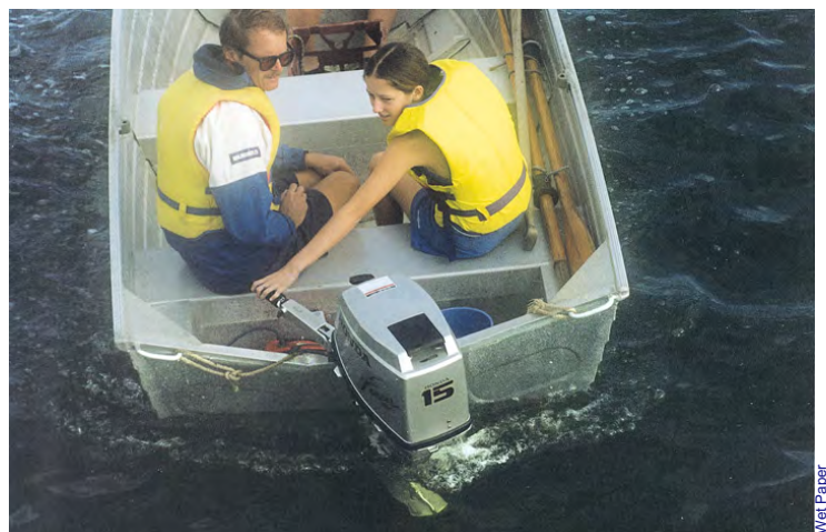
Figure 34.2 Point the motor in the direction you wish to go on reverse
