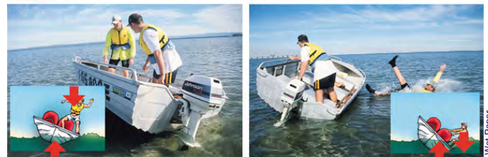
Figure 22.1 If the centre of gravity is lower than the centre of buoyancy, the boat will tip and fill with water
