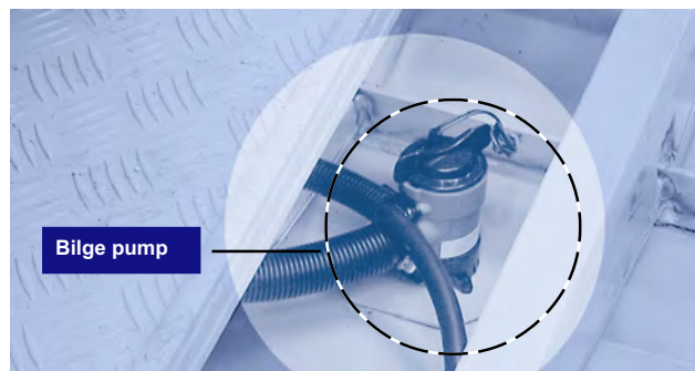
Figure 24.1 A bilge pump is located under the deck and can be operated manually or electrically.
