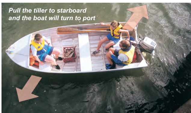
Figure 13.3 Pull the tiller to the right and the boat will turn to port.
