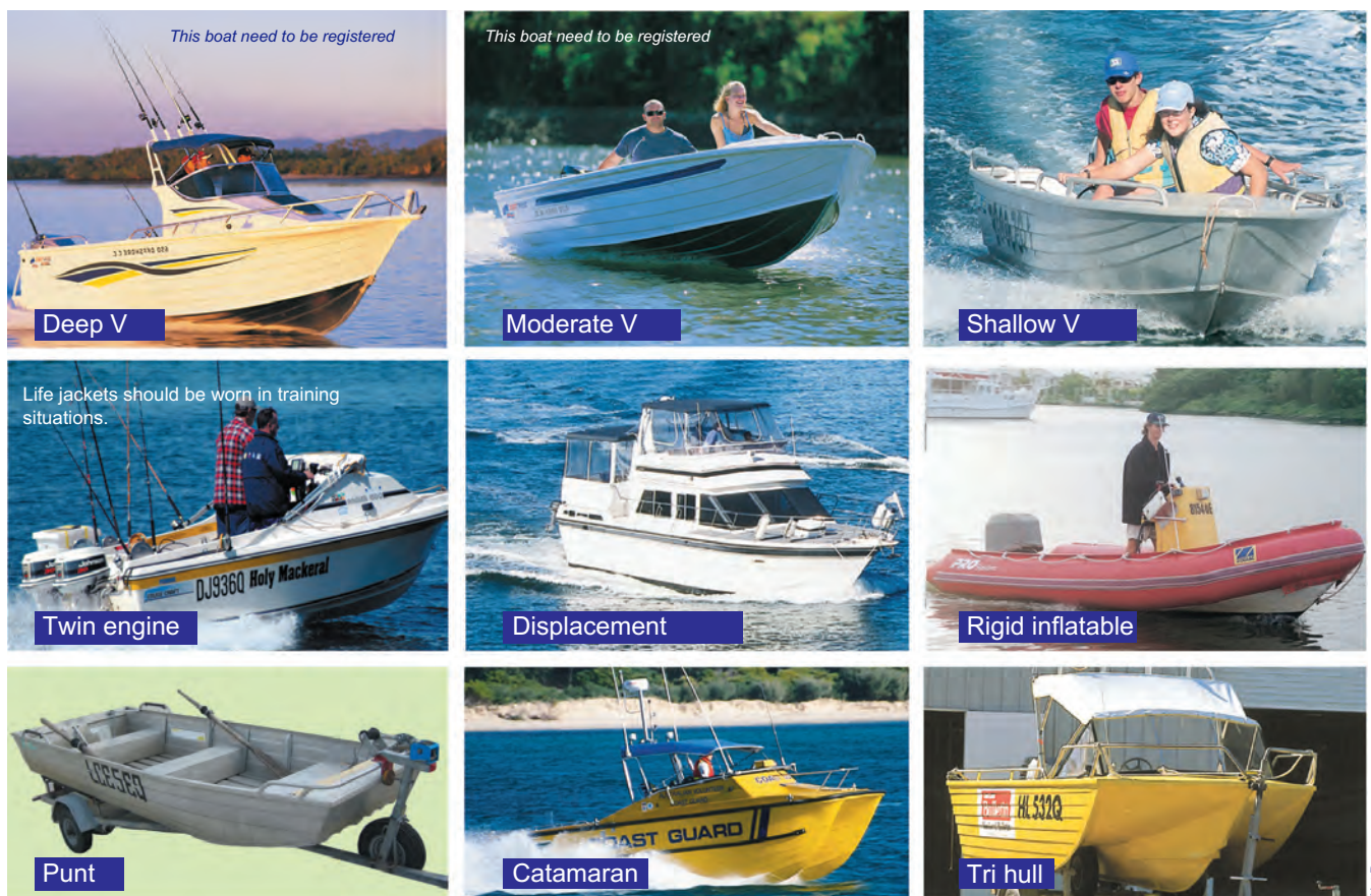
Figure 9.1 Some hull types (Note: In training situations life jackets should be worn by all occupants)
