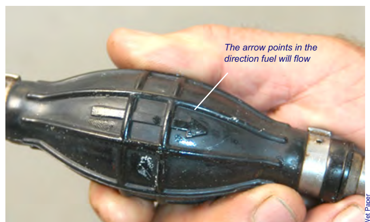
Figure 21.4 Check fuel lines for any leaks.
