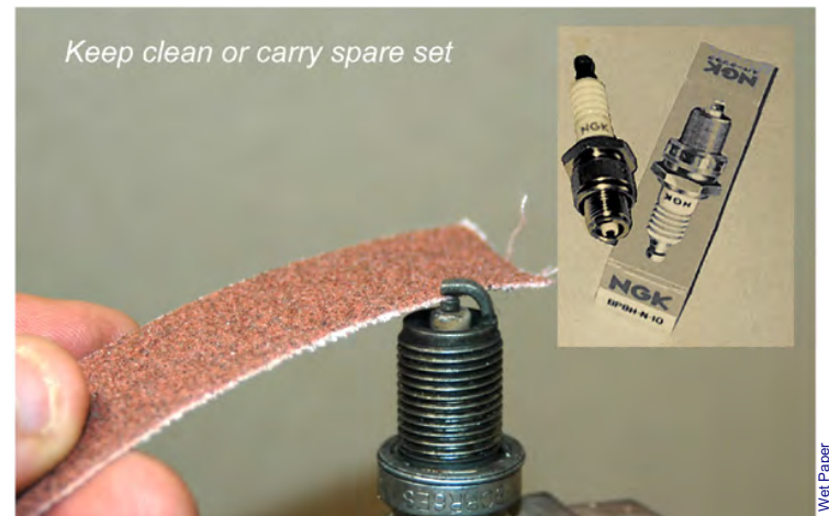
Figure 21.2 Check the spark plug gap and condition.
