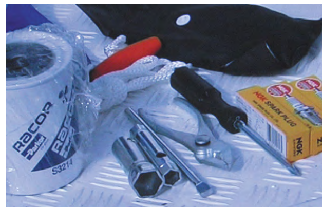
Figure 24.2 Basic tools include spark plug spanner, multi-grips, screw driver, water repellent, fuel filter, emery paper, emergency starter cord
