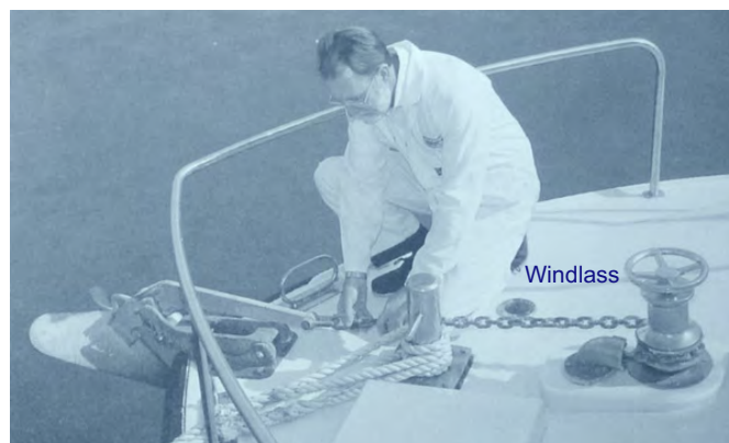
Figure 91.5 Anchor windlass and anchor system on larger boat
