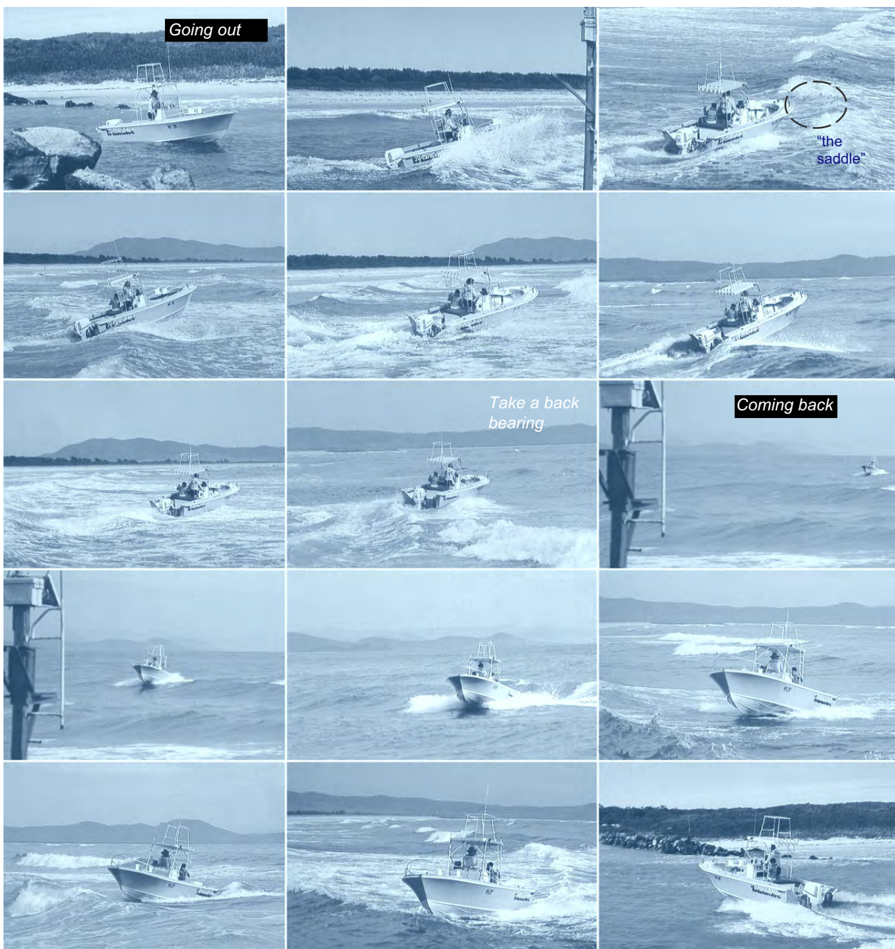
Figure 110.1 Hazards and conditions when navigating a bar (from Safe Boating in Australia by Neil and Young)
