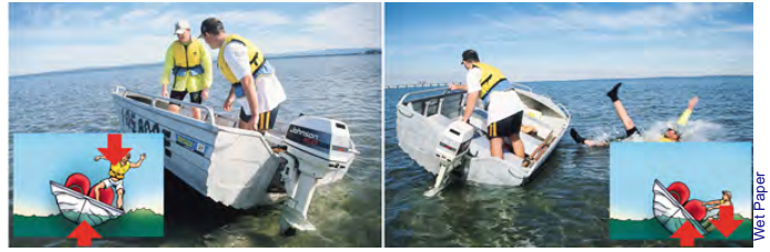
Figure 8.2 Dinghy with enough freeboard to enable it to return to the upright position.
