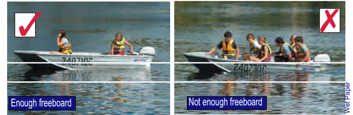
Figure 8.3 An overloaded boat has reduced freeboard
