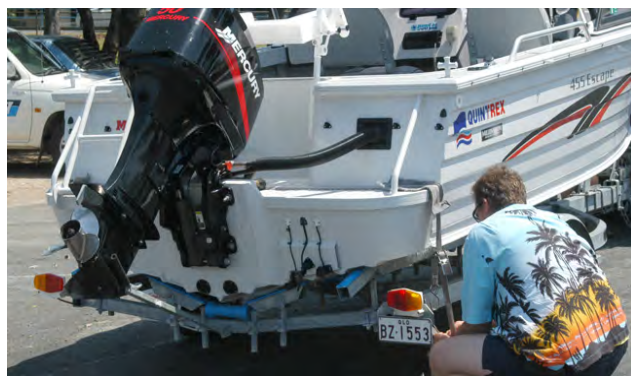
Figure 5.1 Check the lights and allow the bearings to cool.
