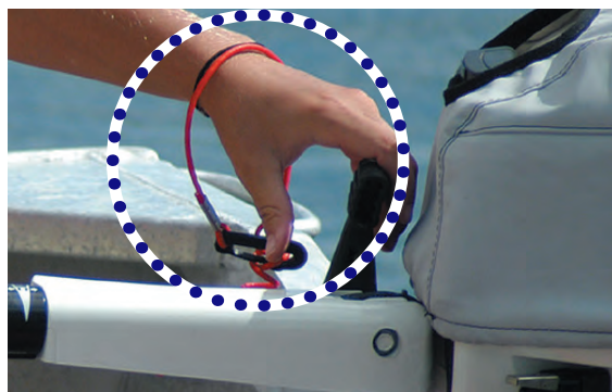
Figure 31.4 Check the safety lanyard (kill switch) is on your wrist .
