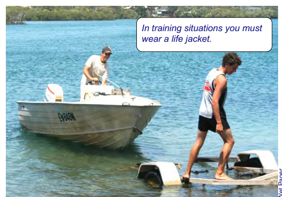
Figure 29.2 Correct launch of trailer
