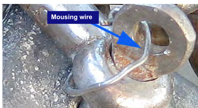
Figure 20.4 Shackles are moused whenever there is a chance of the shackle pin working loose.
