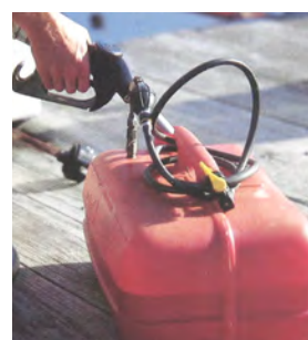
Figure 22.4 Refuelling away from the boat in a well ventilated area
